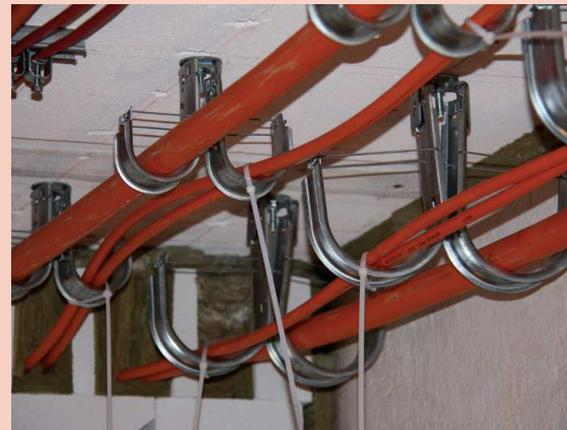
*J-Hooks and cables in fire chamber before fire test*
