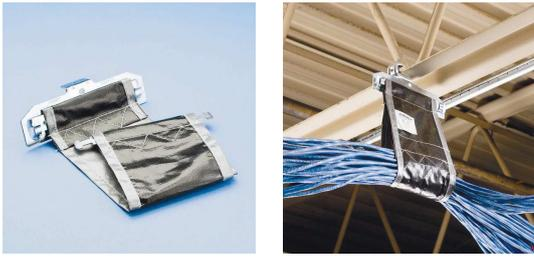
Cat 425 Adjustable Cable Supports provide an ideal solution for retrofit applications in existing facilities where space is limited and cable tray would be very difficult to install. The system supports a large quantity of cable, and can be mounted to overhead building structure or wall-mounted for low-profile installations. The fabric is strong yet flexible, and is suitable for pulling cable.
