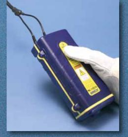
Press and hold operate button. Open mold after
