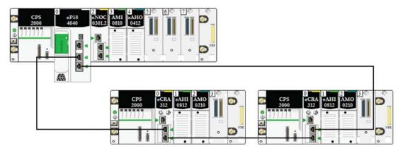
These restrictions apply to the simple daisy-chain loop topology above (which consists of only the local rack and RIO drops):
