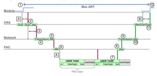
**NOTE:** Overhead in the previous illustration refers to the time period between the end of USER TASK processing (noted by the end of **out**) and the start of the next period (based on CPU USER TASK cycle time).
