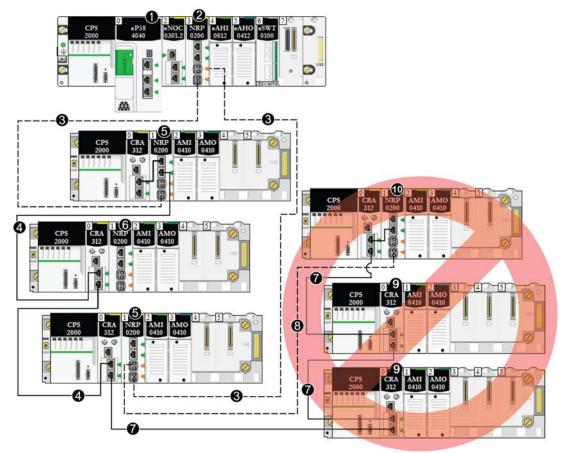
You cannot use BMXNRP020• modules to connect sub-rings to the main ring:
