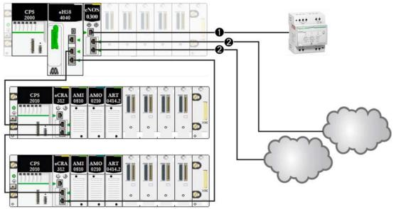
1 The BMENOS0300 module on the local rack is connected to a DIO daisy chain.
