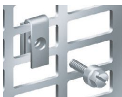
Direct mounting of equipment on nuts.
