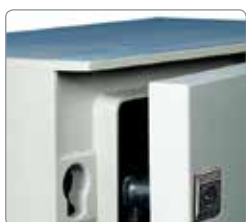
Built-in canopy protecting the door and the sealing gasket. Two double-bar 3-mm (0.1 in.) locks outside the sealed zone.
