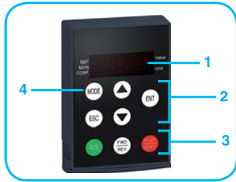
Remote display terminal with cover off
