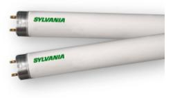
General32W, 48in MOL, T8 OCTRON Extended Value XV fluorescent lamp, 5000KDescription:color temperature, rare earth phosphor, 81 CRI, suitable for RS or IS operation,<br/>ECOLOGIC
