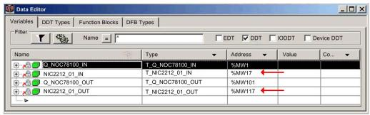
Notice the address locations of the remote EtherNet/IP device's inputs (%MW17) and outputs (%MW117). As you will see, below, when the local slave is activated, these address locations will change.
