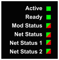
**NOTE:** The Net Status 1 and Net Status 2 LEDs are not functional for the 140NOC78000 distributed I/O head module.
