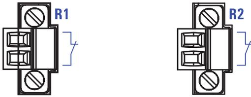
Figure 3: Pin assignment of the signal contact
