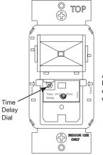
Adjustment controls are located behind the front cover of the unit and are clearly labeled.
