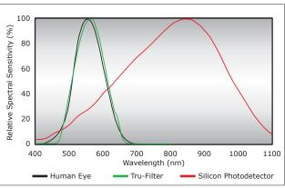
Tru-Filter® spectral sensitivity matches that of the Human Eye; while competitor's Silicon Photodetector comes nowhere close.
