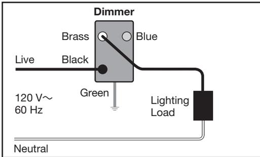
**Note:** Dimmer can be installed on the line side or load side of the circuit.
