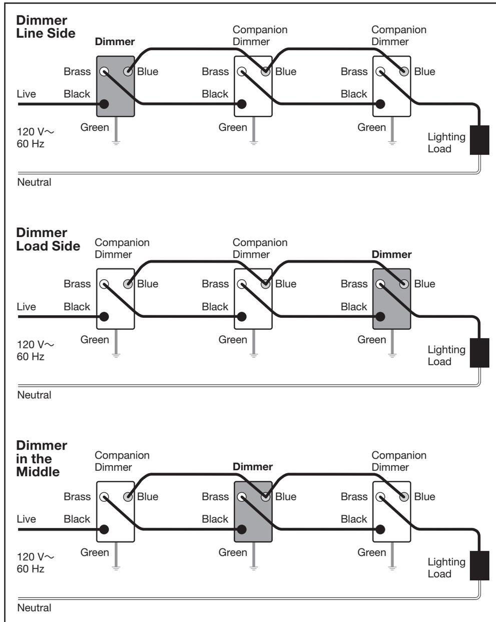
**Note:** Dimmer can be installed on the line side, load side, or in the middle of the circuit.
