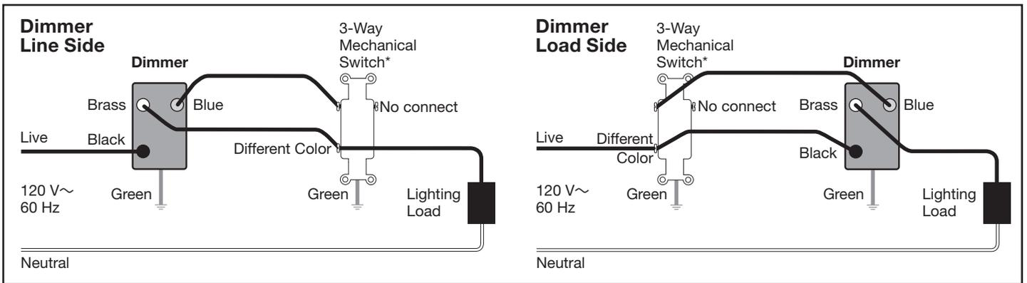
\*Note: Screw terminal positions on 3-way mechanical switches may vary.
