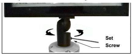
**NOTE:** Swivel stem must be installed with the mounting threads facing down-to-horizontal. Fixtures may not be installed with mounting threads facing upward unless shielded from rain or sprinklers.
