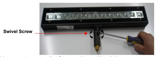
5. Loosen set screw to adjust fixture rotation, and then tighten set screw.
