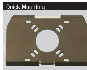
Quick Mounting Quick-mount – easy mounting without opening fixture. Attach adapter plate to wall, connect wires, hang fixture and tighten set screws.
