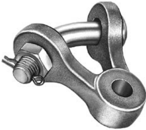
Y-Clevis Eye, Rotated, Ductile Iron, 0.875" Curved Bolt, Eye: 1.125" with 0.813" Hole, UTS 40,000 lb
