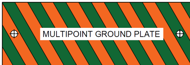
FAA3 = MULTIPOINT GROUND PLATE* Alternating Green and Orange stripes
