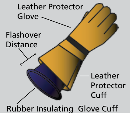
CLEARANCE (FLASHOVER DISTANCE) TABLE PER ASTM F496
