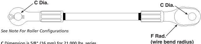
C Dimension is 5/8" (16 mm) for 21,000 lbs. series D Dimension is 0.9" (23 mm) for 21,000 lbs. series E Dimension is 1.4" (36 mm) for 21,000 lbs. series
