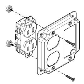
Note: If you do not see the perforation it might be necessary to snip the pieces off with a cutting tool. Avoid removing too much strap to maintain the integrity of the device mounting holes.
