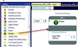
The Restart Function requires a leading and trailing edge within a specific time frame. The pulse width must be between 250...3000 ms. If the pulse width is too short or too long, the Restart function is not executed.
