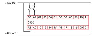
Figure 87 - Example Schematic for 2 N.C. with Two Test Pulses Sources
