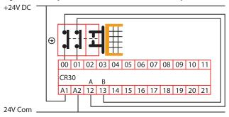
Figure 45 - Example Schematic of a Dual Channel Safety Gate Switch Using OSSD Outputs
