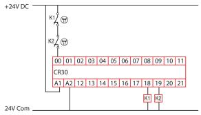
Figure 41 - Example Feedback Schematic with Four Feedback Contacts Connected Individually to Four Input Terminals
