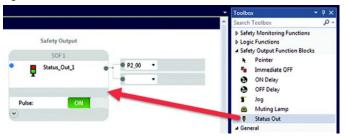
See <u>Figure 74</u> (page 76) and <u>Figure 75</u> (page 77) for examples of how the Status Out block works with the Status In block. <u>Figure 73</u> (page 76) shows how the Status Out block is used with other functions. In this example, the Status\_Out\_1 block pulses its output as soon as the E-stop button is pressed. When the E-stop button is released, the Status\_Out\_1 block turns OFF.
