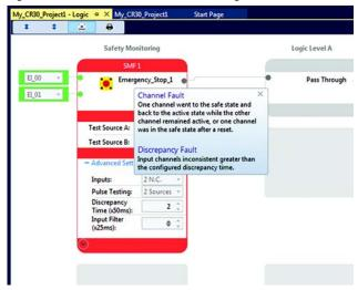
The type of fault is also shown in the top panel of the Project tab (Figure 143).
