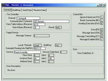
**2.** Set the Ethernet network address of the Guardmaster 440C-ENET plug-in module as the target of the message instruction:
