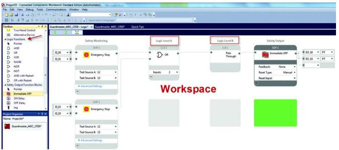
Figure 97 - Logic Levels A and B on the Connected Components Workbench Workspace
