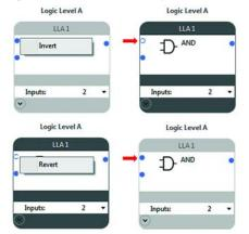
Figure 111 - Invert or Revert Input Connection Points
