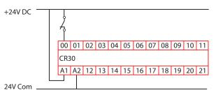
Figure 84 - Example Schematic for Single-Channel N.C. with Test Pulse
