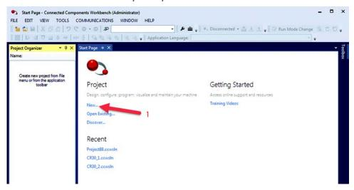
The Connected Components Workbench software maintains a list of projects to help prevent you from overwriting an existing project. The name of each new project increments by one (for example, Project90). This window allows you to select a name and a location for the file.
