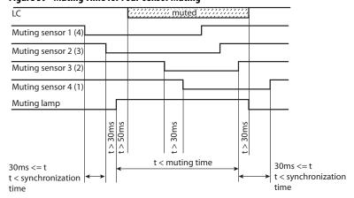
Figure 59 - Muting Time for Four-sensor Muting
