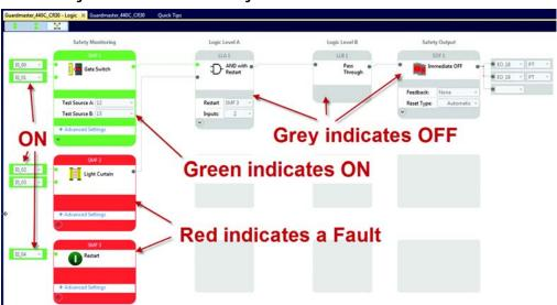
Mouse over the red block, and the Connected Components Workbench software displays an error message for 5 seconds. Move the mouse away and then back over the block to show the message again. The fault tooltip automatically appears once a fault is detected during the online monitoring mode. You can acknowledge the
