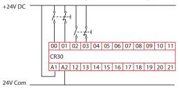
When test pulses are used, the CR30 safety relay will detect a short from Channel 1 to Channel 2 after 3.7 seconds and turn the output OFF. To clear the fault, release both buttons.
