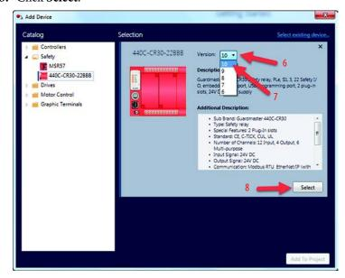
TIP To determine the current firmware revision, open RSLinx, right-click the CR30 safety relay, and click **Device Properties**.
