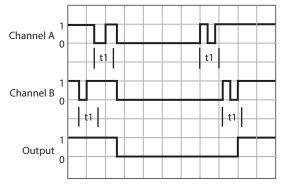
Input filtering can set in 25-ms increments, from 0...1000 ms. The default value is 0 ms.
