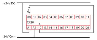
Figure 85 - Example Schematic for Single Channel OSSD
