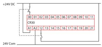
Figure 90 - Example Schematic for N.C./N.O. with One Test Pulse
