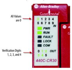
If the CR30 safety relay configuration has been verified, pressing the **Verification** button cycles the status indicators through each verification digit. In <u>Figure 15</u>...<u>Figure 18</u>, the Verification ID is 7916.
