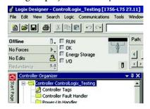
For ControlLogix users who want to add a Guardmaster 440C safety relay online manually, go online with the ControlLogix controller using RSLogix 5000 or Studio 5000 Logix Designer application. The ControlLogix controller can be in Remote Run or Program mode.
