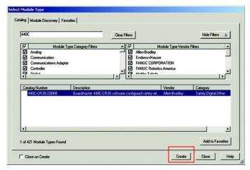
If the Guardmaster 440C safety relay is not shown, go to <a href="http://www.rockwellautomation.com/global/support/pcdc.page">http://www.rockwellautomation.com/global/support/pcdc.page</a> and download the latest RSLogix 5000 safety relay Add-on Profile. Add-on Profile version 2.01 (or later) includes support for the embedded configuration editor.
