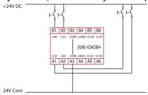
Figure 123 - 2080-IQ40B4 Schematic Showing Four Standard Output Signals
