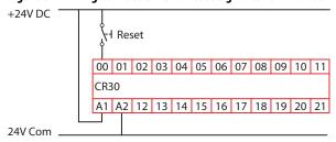
The reset block works with one or more output blocks. When an output block requires a manual reset, the Connected Components Workbench software shows all available reset inputs that can be used.
