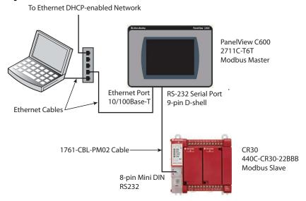
In <u>Figure 134</u>, a Micro830\* programmable logic controller (PLC) is connected to the CR30 safety relay by the 8-pin DIN serial port connections. The Micro830 PLC can read/use status information from the CR30 safety relay and can send reset and restart signals to the CR30 safety relay.
