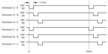
The purpose of the test pulses is to detect short circuits from the input signal to 24V DC, 24V common, and shorts from one input signal to another input signal. If one input signal is assigned to Test Pulse A and another signal is assigned to
