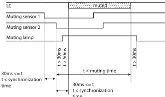
Figure 56 - Muting Time for Two-sensor L-type Muting
