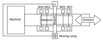
The material can travel in either direction; breaking MS1 first and MS4 last or breaking MS4 first and MS1 last. The muting lamp turns on and the light curtain is muted after the second sensor is blocked. The object must be large enough to break all four sensors.
