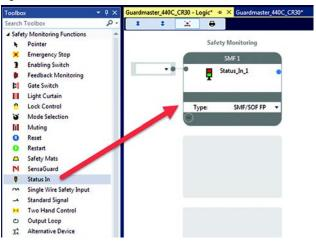
**Ready-for-reset** - In the Type field, select the **SOF RR** option. Then, assign an input to the desired Safety Output block.
