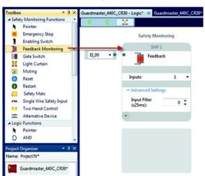
Figure 39 - Feedback Monitoring Function Block
