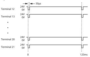
Then a sequence occurs in which each output is individually tested twice. The test pulse is  $50~\mu s$  wide. The test pulses occur every 250~ms and switch to the next output configured with testing.
