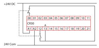
Figure 91 - Example Schematic for N.C./N.O. with Two Test Pulses
