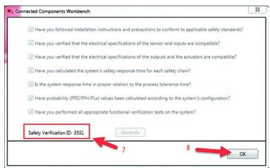
The ID is stored in the CR30 safety relay. During power-up, the CR30 safety relay uses this number during its self-testing to verify that its internal processors are functioning properly. When the configuration is uploaded from the CR30 safety relay, the Connected Component Workbench software shows the Verification ID.
