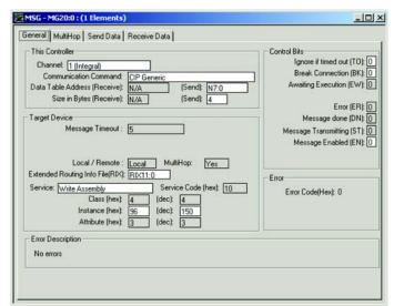
2. Set the Ethernet network address of the Guardmaster 440C-ENET plug-in module as the target of the message instruction.
