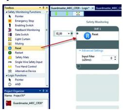
To help prevent inadvertent actuation of the reset block, the reset requires a leading and trailing edge within a specific time frame. The pulse width must be
