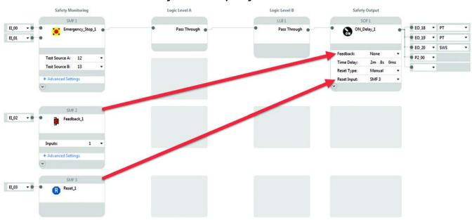
Figure 115 - ON Delay Configuration
