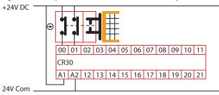
Figure 44 - Example Schematic of a Dual Channel Safety Gate Switch Using Test Pulses A and B
