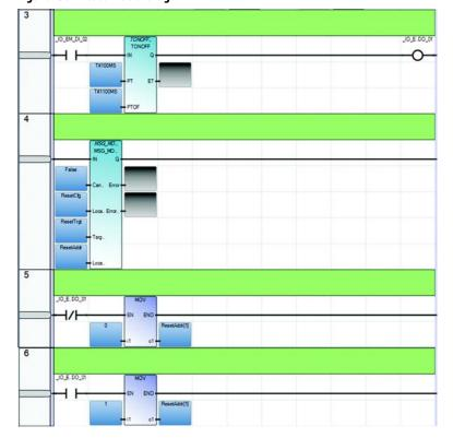
Figure 138 - Reset Ladder Diagram
