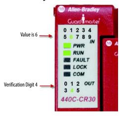
After 5 seconds, the status indicator will revert to show the status of the inputs and outputs as configured in the Connected Components Workbench software.
