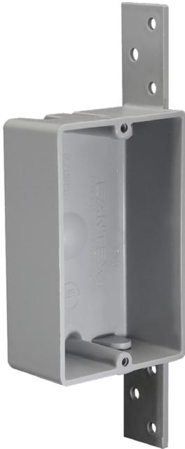
CANTEX EZ08SB is a 1-gang, 8 cubic inch, PVC switch or outlet box that is great for residential and light commercial new construction (new work) applications where a shallow electrical box is needed. It features a molded-on PVC bracket for easy mounting on wood or metal studs.
