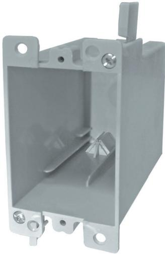
EZ21SO EZ BOX is a 1-Gang, 21 cu. in., renovation application (old work) electrical switch or outlet box for residential or light commercial renovation (old work) projects when a 1-gang box is needed. EZ mount flanges, winged swing tabs and 4 built-in, contractor preferred v-clamps make installation easy and cost effective.
