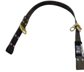
1200110 CYNCH-LOK REPLACEMENT STRAP FOR DISTRIBUTION POLES POLE SIZE (DIA/CIRC): MIN. .1 M/1.5 M (5.5"/17.5") MAX. .5 M/1.5 M (18.5"/58") DURABLE STRAP WITH WEAR INDICATOR, STOPPING CLEAT, FIELD REPLACEABLE STRAPS
