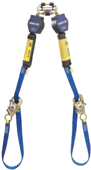
3101378 NANO-LOK™ TIE-BACK SRL TWIN LEG 2268 KG (5,000-LB.) GATED SNAP HOOK WITH TWIN LEG QUICK CONNECTOR, 2.7 M (9')
