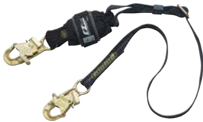
1246317 EZ-STOP FORCE2 ADJUSTABLE SHOCK ABSORBING LANYARD ..... 1.8 M (6') ADJUSTABLE WEB SINGLE-LEG FORCE2 WITH NOMEX®/KEVLAR® FIBER WEB AND SHOCK PACK, SNAP HOOKS AT EACH END
