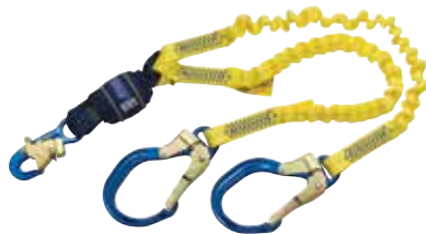
1246145 EZ-STOP FORCE2 WRAPBAX ELASTIC WEB ..... 100% TIE-OFF ALUMINUM SNAP HOOK AT ONE END, ALUMINUM REBAR (64 MM (2.5") GATE OPENING) AT LEG ENDS X 1.8 M (6')
