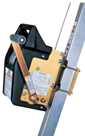
8102001 SALALIFT II WINCH WITH 60' (18.3 M) OF 1/4" (6.4 MM) GALVANIZED CABLE, MOUNTING BRACKET AND WINCH BAG
