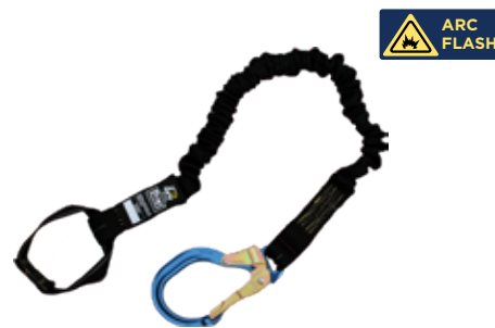
1244614 SHOCKWAVE2 ARC FLASH 6' (1.8M) SINGLE LEG WITH NOMEX®/KEVLAR® FIBER WEB, CHOKER ON ONE & ALUMINUM REBAR HOOK ON LEG END. ASTM F887
