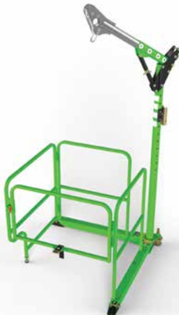
8530352 ADVANCED 4-IN-1 DAVIT GUARD SYSTEM PORTABLE FALL ARREST, CONFINED SPACE ENTRY AND RESCUE SYSTEM WITH DAVIT AND GUARDRAIL. SYSTEM INCLUDES A COLLAPSIBLE BASE TO REDUCE STORAGE AND TRANSPORT SPACE. A STANDARD TIE-OFF POINT PROVIDES A CONVENIENT 5000 LB. (22KN) ANCHORE POINT FOR FALL ARREST DEVICES WHERE REQUIRED. INCLUDES WINCH-MOUNTING BRACKET
