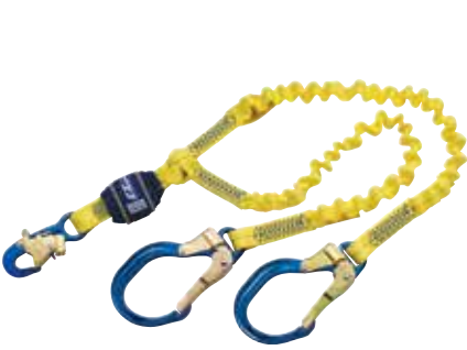
1246193 EZ-STOP ELASTIC WEB LANYARD 100% TIE-OFF ALUMINUM SNAP HOOK AT ONE END, ALUMINUM REBAR (2.5" (64 MM) GATE OPENING) AT LEG ENDS X 6' (1.8 M)
