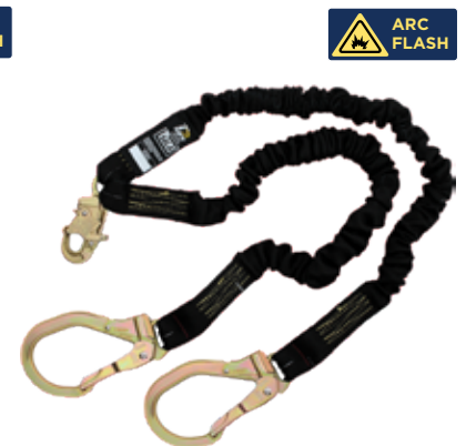
1244633 SHOCKWAVE2 ARC FLASH 100% TIE-OFF SNAP HOOK AT ONE END, STEEL REBAR (2.5" (64 MM) GATE OPENING) AT LEG ENDS X 6' (1.8 M) NOMEX®/KEVLAR® FIBER, ELASTIC LEGS. ASTM F887
