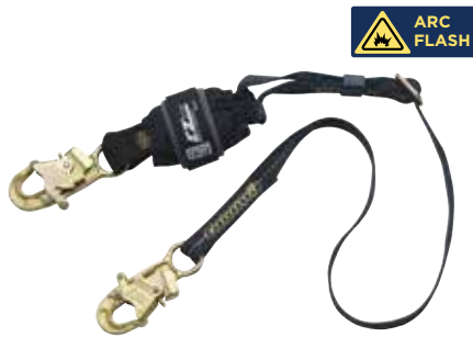
1246317 EZ-STOP FORCE2 ARC FLASH ADJUSTABLE SHOCK ABSORBING LANYARD 6' (1.8 M) ADJUSTABLE WEB SINGLE-LEG FORCE2 WITH NOMEX®/KEVLAR® FIBER WEB AND SHOCK PACK, SNAP HOOKS AT EACH END ARC FLASH ASTM F887
