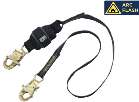
1246306 EZ-STOP ARC FLASH SHOCK ABSORBING LANYARD 6' (1.8 M) WEB SINGLE-LEG WITH NOMEX®/KEVLAR® FIBER WEB AND SHOCK PACK, SNAP HOOKS AT EACH END ASTM F887
