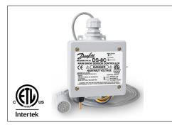
The DS-8C controller is designed for roof and gutter and snow melting applications. It senses both moisture and temperature conditions in the gutter or down spouts. The sealed low voltage, remote mount precipitation sensor can be mounted in a down spout, on the back of a gutter, under the drip edge, up to 10 feet away, while keeping the main controller in a more convenient and protected location.
