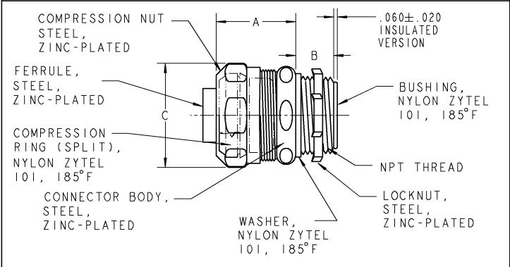
3/8" TO 2" TUBULAR STEEL CONNECTORS, SEE SHEET 2 FOR SIZES 2-1/2" TO 4".
