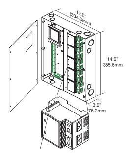
Modules clip onto DIN rail, and plug to panel power supply and each other via integral connectors.
