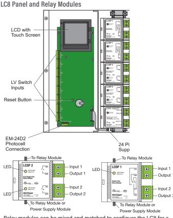
Relay modules can be mixed and matched to configure the LC8 for a variety of single-pole and double-pole lighting control applications.
