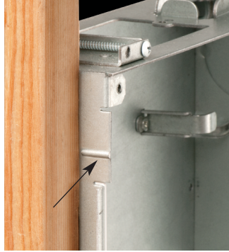
Positioning tabs are set for 1/2" or 5/8" drywall.
