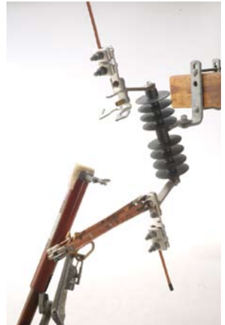
Loadbreak tool disconnected from loadbreak hook and ready to be disconnected from blade pull ring
