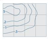
**Vertical Lamp Perimaliter®** – Wide lateral spacings 6 times mounting height for 1 FC mininum between fixtures
