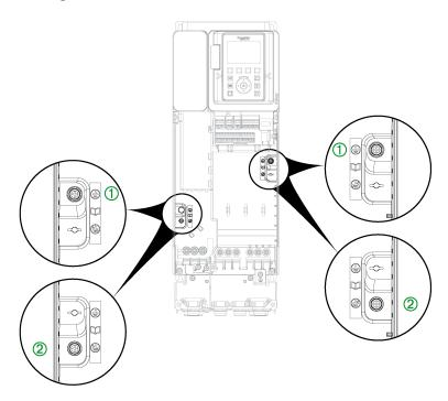
Setting For Frame Size 3S, Frame Size 3Y and Frame Size 4 Products, 200...240  $\mbox{\ensuremath{V}}$
