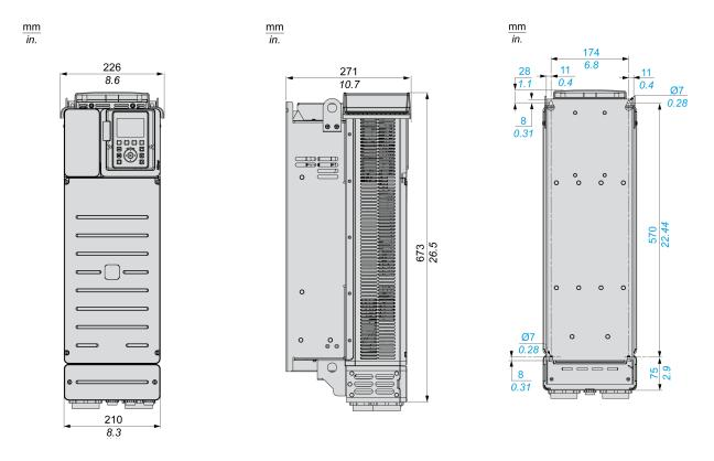
IP20 Drives, except on Lower Part (IP00) - Front, Side And Rear View
