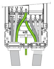
**NOTE:** PA/+ and PC/- terminals are used only to measure the DC Bus voltage and are not intended to be wired for an external use.
