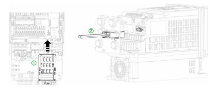
To help ensure correct wiring of the control part, apply the following instructions to install the PROFIBUS fieldbus module on Frame size 1 drives
