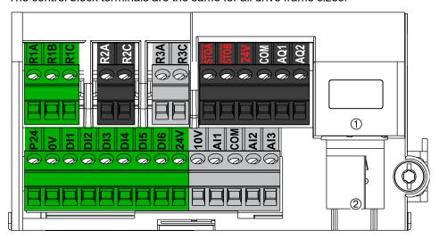
1 Ethernet Modbus TCP, 2 Serial Modbus
