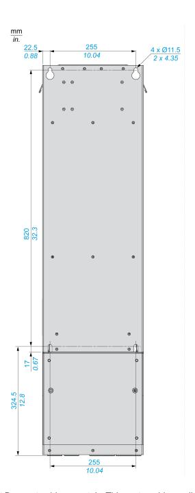
**NOTE:** Lower Conduit Box part sold separately. This part enables wall mounting of the product. It provides IP21 protection degree on the bottom side and UL type 1 protection degree.
