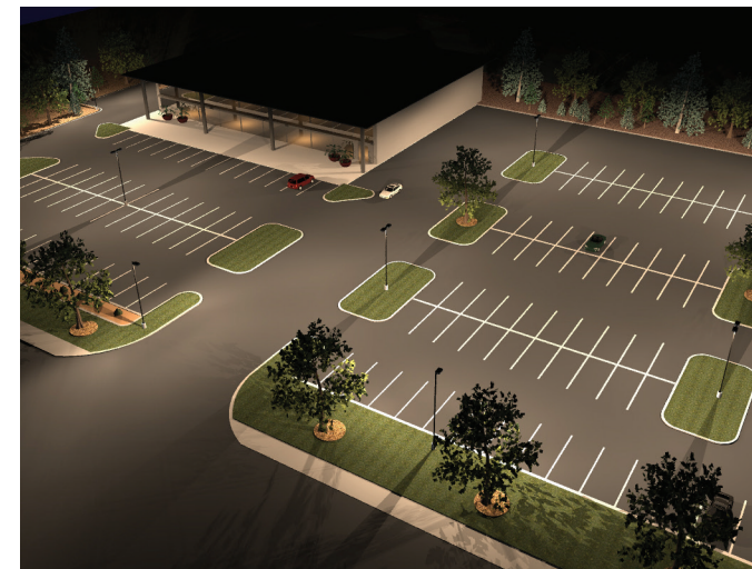
Prevail A40 LED 14 Fixtures = 2,002 Total watts
