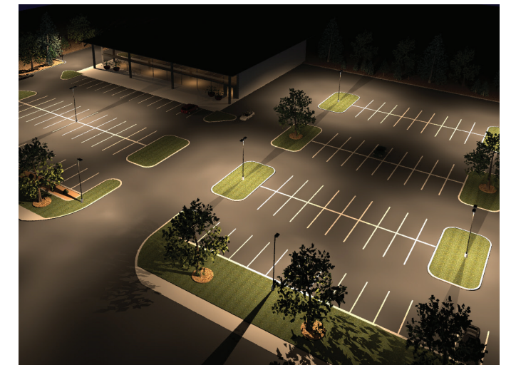
400W Pulse Start Metal Halide 14 Fixtures = 6,370 Total watts
