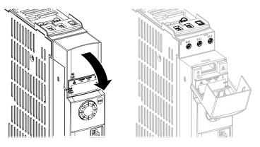
Apply the following instructions to access the power terminals on **frame sizes 1B** and **2B** drives:
