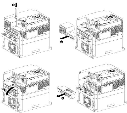
Apply the following instructions to access the power terminals on **frame sizes 3C** drives:
