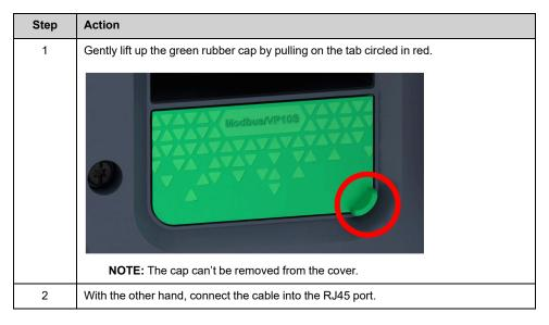
Perform the following instructions when removing the cable from the RJ45 port.
