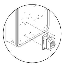
These drives can be equipped with an optional GV2 circuit-breaker, using the optional base plate VW3A9922 and rotary handle GVAPB65S, supplied with detailed mounting instruction sheet PHA63344.
