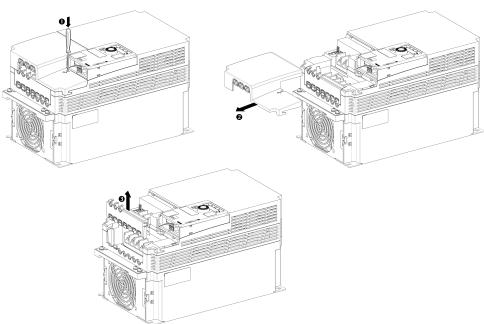
Apply the following instructions to access the power terminals on **frame sizes 5C** drives:
