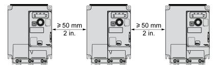
Free space ≥ 50 mm (2 in.) on each side, with vent cover fitted.
