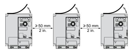
Free space  $\geq$  50 mm (2 in.) on each side. Vent cover should be removed for operation at surrounding air temperature above 50 °C (122 °F). The degree of protection becomes IP20.
