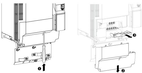
Apply the following instructions to access the power terminals on **frame sizes 4B** and **5B** drives:
