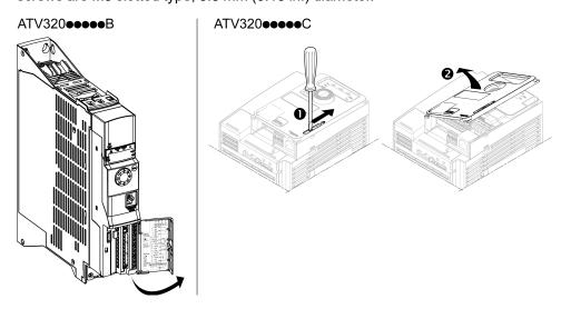
Control block of ATV320•••••C and ATV320•••••W(S) can be removed to facilitate the wiring.
