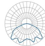
This graphic representation illustrates the LED optical fine-tuning range that Cree can provide. The gray area represents Type V Short optic coverage used to comply with more stringent light spill and high angle brightness specifications or codes by incorporating a lower main beam. The extended blue area indicates the Type V Medium optic coverage that uses a slightly higher main beam to allow wider, more economical pole spacing.
