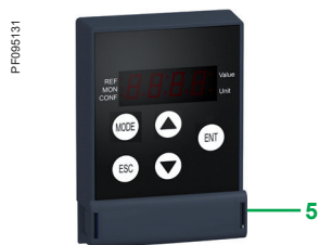
Remote display terminal with cover closed
