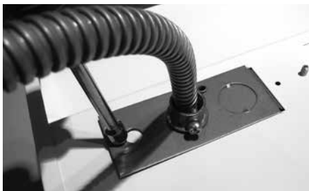
Step 4 Reinstall the knock out plate.
