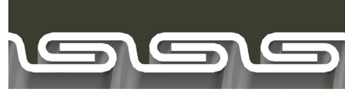
Interlocked Design 1-1/2" through 4" with no bonding wire
