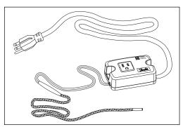
The RX1200 controller is designed to use in conjunction with Danfoss roof and gutter de-icing cable for roof, gutter and snow melting applications. The RX1200 sense both moisture and temperature conditions in the gutter or downspouts and turns the roof de-icing cable on and off based upon these readings.
