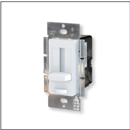
NEXUS® All-in-One LED Driver and Dimmer NATL-SWEX60/24A 24V 60W NATL-SWEX100/24A 24V 100W Input Voltage: 120V Dimming: Integral Dimmer Description: Eliminates the driver and allows 120V input and 24V output from a single gang box. 100-5% dimming and on/off switch.
