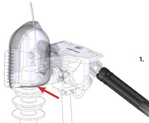
1. Using the hotstick holes on the cutout guard, pull it over the top skirt of the insulator. Ensure the conductor is routed up and out, and only the top skirt is inside the guard, as shown.
