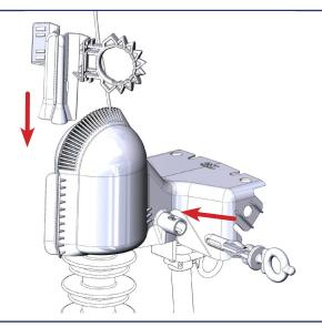
2. Using the included hotstick spur, apply the wedge clip to front of the cutout guard, pulling it down until fully engaged. Insert pin into either side, ensuring it inserts below the cutout's top hood. Fully seat the pin with a firm push.
