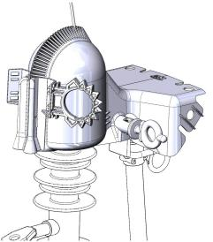
**3.** Ensure cutout guard is secured by testing movement with rear hotstick holes. Installation is complete.
