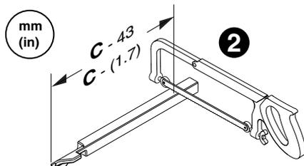
**Typical Operating Shaft Installation**
