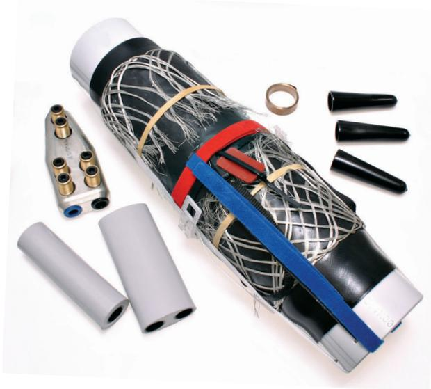
Prysmian has expanded its cold shrink technology to include a live end cap. This provides the customer the flexibility of installing medium voltage cable that can be fully energized but spliced or terminated at a later time. Typically this is performed after a MV Branch Joint where the extra cable end is not ready within the network to carry load.
