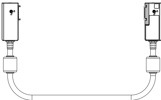
5094-CE05, 5094-CE10, 5094-CE30 With fixed ferrite core
