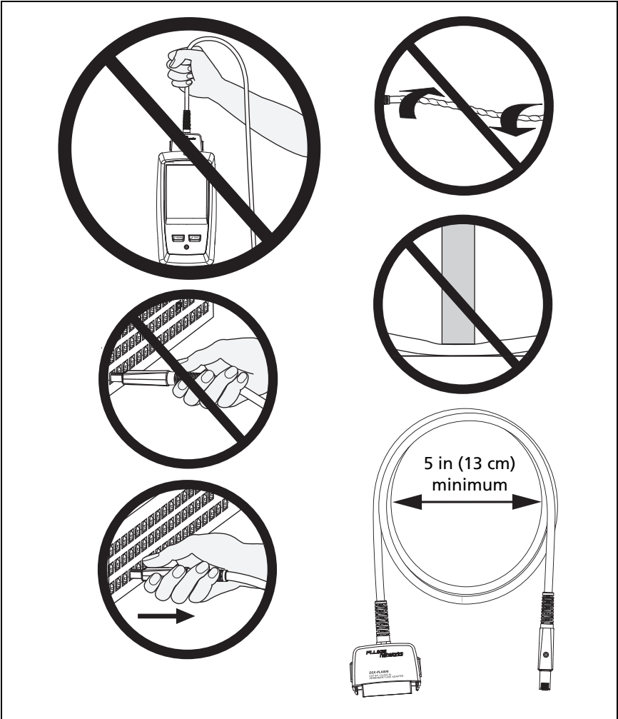
Figure 10. How to Prevent Damage to the Permanent Link Adapter Cables
