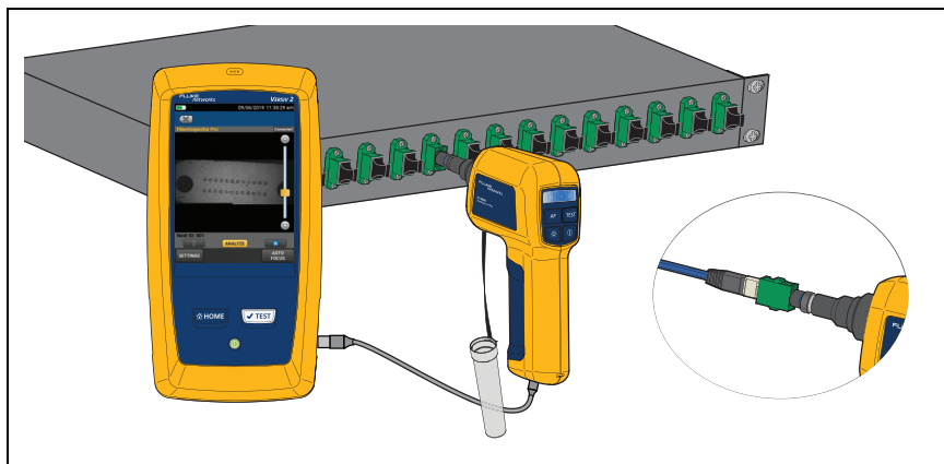
Figure 48. Inspect an Endface (FI-3000 shown)
