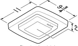
Dimensions shown in inches. Compatible with existing fan housing dimension of  $7 \ensuremath{\,^{\!\!\!/}_{\!\!\!\!\!\!2}}$  " x $7\frac{1}{4}$ " and  $8\frac{1}{4}$ " x 8". See chart above for specific models.
