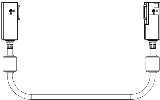
5094-CE05, 5094-CE10, 5094-CE30 With fixed ferrite core
