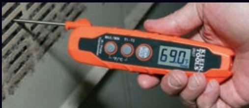
Probe accurately measures air, liquid, and surface temperatures, -40 to 572°F (-40 to 300°C)
