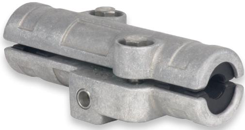
The HIBUS Series Conductor Trunnion is designed to reduce static and dynamic stress at the attachment point on transmission conductors without the use of armor rods or line guards. Rated for 250°C operation, the HIBUS Series Conductor Trunnion has a specially formulated bushing material for high temperature conductors.
