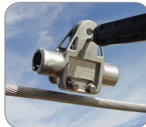
3. With the HIBUS Suspension in the open position, locate the "Hot Stick" (with Live-line Attachment Tool attached) on the conductor
