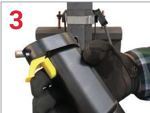
3 Release the control unit trigger guard, press and hold the switch and wait for the ignition.
