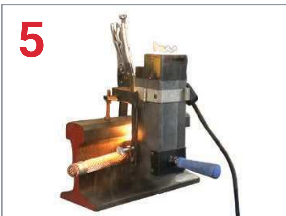
5 After reaction, open the mold and remove the expended steel cup – no special disposal required.
