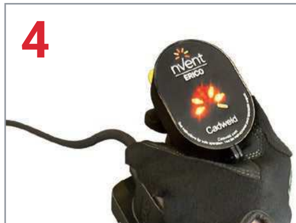
3 Release the control unit trigger guard, press and hold the switch and wait for the ignition.
