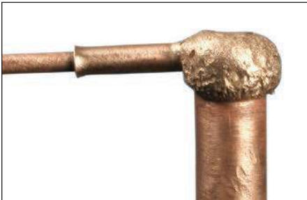
Fig. 16 – You are ready to make another Cadweld connection.
