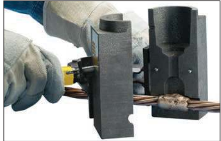
Fig. 28 – Open the mold and remove the connection. Use care to prevent chipping the mold. Avoid contact with hot materials. See the “Cadweld Quality Standards” section to see whether a quality connection has been made.
