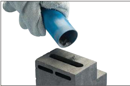
Fig. 23 – Close the lid and pour the remaining 3/4 to 2/3 of the starting material into the slot on the mold cover.
