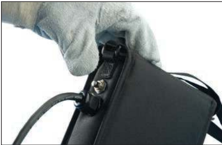
Fig. 26 – Using the Cadweld Exolon battery pack, press the button. At this time, the unit will send a charge to the igniter pin. The igniter pin will initiate the Cadweld Exolon exothermic reaction.
