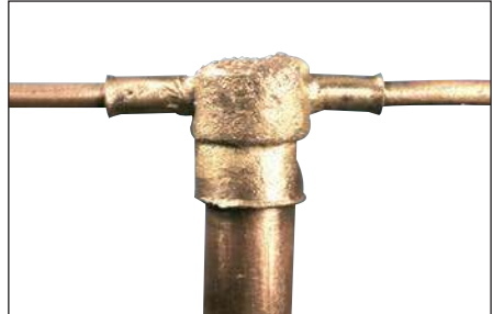
Fig. 17 – You are ready to make another Cadweld One Shot connection.
