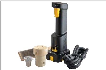
Fig. 2 – Prepare the proper materials and equipment for the type of connection you are making. The Cadweld Plus One Shot system requires a Cadweld One Shot ceramic mold, Cadweld Plus welding material, wire brush for cleaning/preparing conductors, nVent ERICO Cadweld Plus Impulse Exothermic Welding Control Unit, and propane torch.
