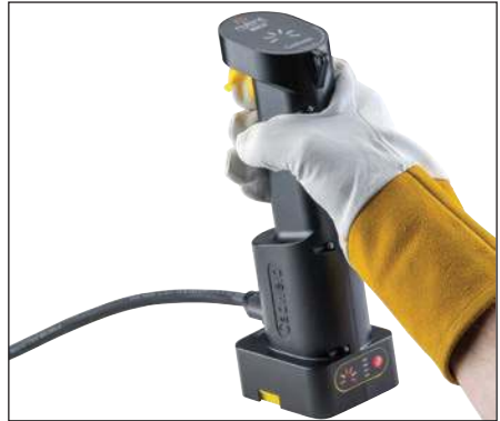
Fig. 13 – Using the control unit, lift the trigger cover and press the ignition button and hold. You will see the 6 lights on the top of the control unit light up as it is charging. After the 6th light is illuminated, the control unit will send a charge to the ignition strip, initiating the Cadweld Plus exothermic reaction. Allow approximately 30 seconds for completion of the reaction and solidification of the molten material.
