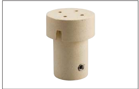
Fig. 3 – Check to ensure the ceramic mold is not worn or broken, which could cause leakage of molten weld metal during the reaction.
