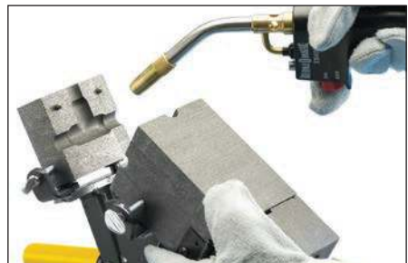
Fig. 10 – Graphite absorbs moisture. Ignite the propane torch and dry out the inside of the mold thoroughly on both sides, heating the mold to approximately 250 degrees Fahrenheit (120 degrees Celsius).
