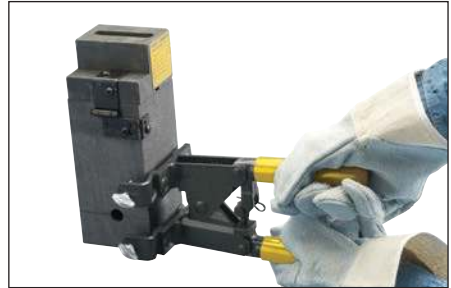
Fig. 8 – Close the grips to tightly lock the mold. Check for an appropriate seal on the mold.
