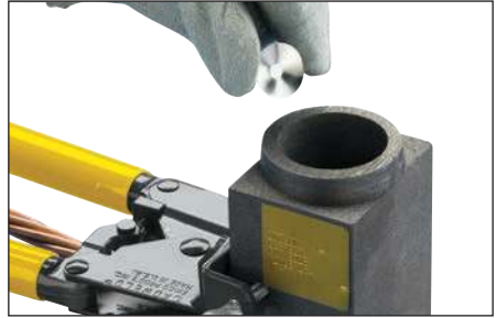
Fig. 18 – Insert the steel disk (concave side up) into the mold. Hold the steel disk on the side of the mold and let it slide into place.
