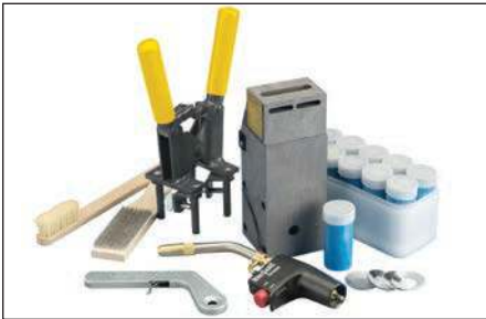
Fig. 2 – Gather the proper materials and equipment for the type of connection you are making. The typical Cadweld system requires a graphite mold, handle clamp, welding material, natural bristle brush for mold cleaning, wire brush for cleaning/preparing conductors, flint igniter, and propane torch.
