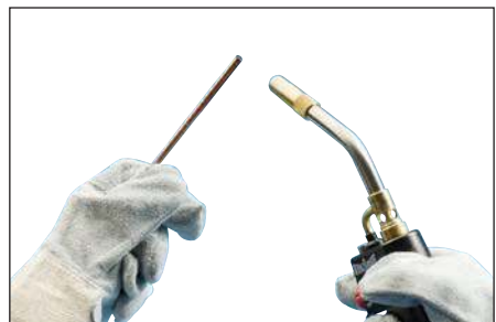
Fig. 4 – The conductors should be clean and dry before the connection is made. Use a propane torch to dry wire conductors and remove remaining cleaning residue, solvent, or water before making the Cadweld One Shot connection.
