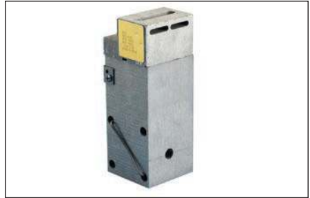
Fig. 3 – Check to ensure the graphite mold is not worn or broken, which could cause leakage of molten weld metal during the reaction.
