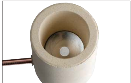
Fig. 9 – Ensure that the steel disk is properly seated inside the Cadweld One Shot.
