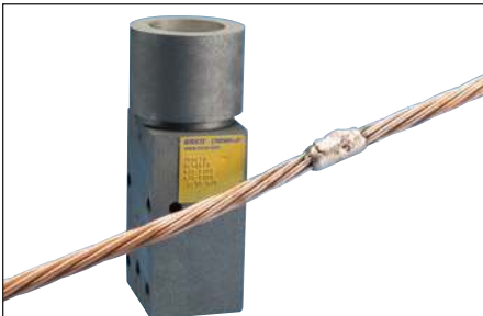
Fig. 31 – Ready to make another Cadweld connection.
