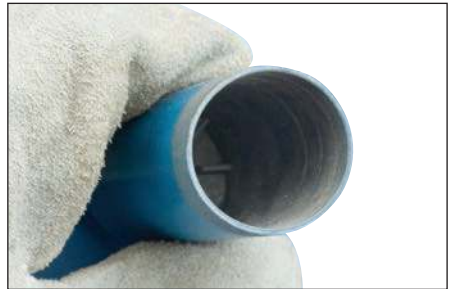
Fig. 21 – The bottom of the tube contains compressed material (starting material). Tap the bottom of the tube a couple of times to loosen this material.
