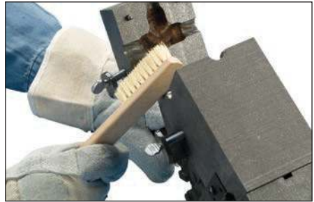
Fig. 24 – Cadweld graphite molds will last for approximately 50 connections. Use a soft cotton cloth or a soft bristle brush (nVent ERICO part #T394) to clean inside the mold cavity and cover.
