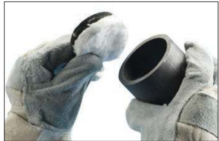
Fig. 14 – Each Exolon package contains 2 filters for a low emission connection. Insert the white ceramic and black graphite filters into the mold cover. (Filters must be changed every 4 connections.)
