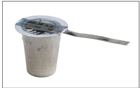
Fig. 8 – Inspect the cup to ensure it is tightly sealed and the ignition strip is securely attached to the seal.
