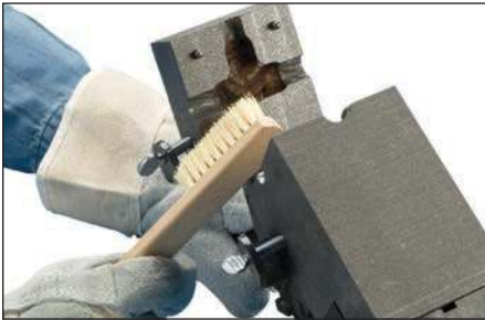
Fig. 27 – Cadweld graphite molds will last for approximately 50 connections. Use a soft cotton cloth or a soft bristle brush (nVent ERICO part #T394) to clean inside the mold cavity and cover.
