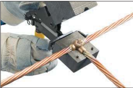
Fig. 22 – Open the mold and remove the connection. Use care to prevent chipping the mold. Avoid contact with hot materials. See the “nVent ERICO Cadweld Quality Standards” section to see whether a quality connection has been made.
