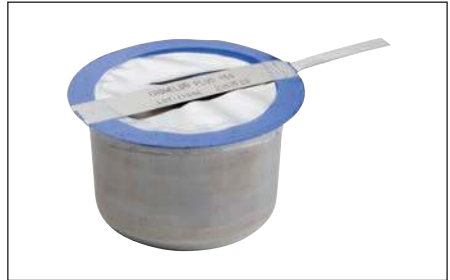
Fig. 15 – Remove the proper Cadweld Plus welding material cup from the plastic container. Inspect the cup to ensure it is tightly sealed and the ignition strip is securely attached to the seal.
