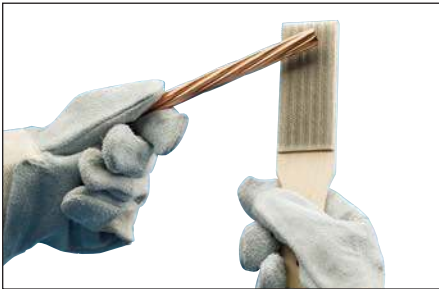
Fig. 12 – Next, use a wire brush to further prepare the surface of the conductors and ground rod (nVent ERICO T-313 or T-314 brush). Scrape the outer surface to remove dirt and oxidation. You will notice a slight color change.
