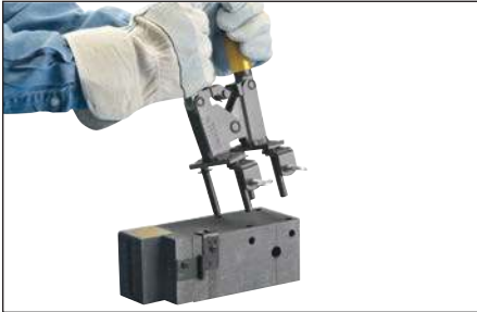
Fig. 6 – Slide the handle clamp into the pre-drilled holes with the proper orientation for the thumbscrews.
