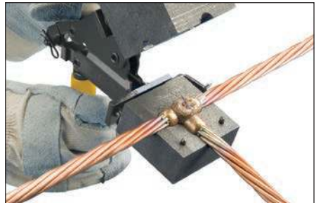
Fig. 25 – Open the mold and remove the connection. Use care to prevent chipping the mold. Avoid contact with hot materials. See the “nVent ERICO Cadweld Quality Standards” section to see whether a quality connection has been made.
