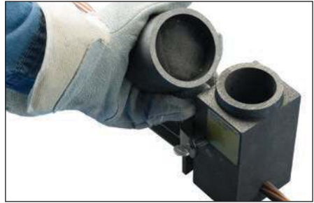
Fig. 27 – Remove the alligator clips from the igniter pin. Remove the graphite cover of the Cadweld Exolon mold.
