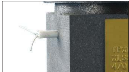
Fig. 23 – Next, take an igniter pin and place it halfway into the small hole on the side of the mold, with the loop side facing into the hole. Spread the wire leads.
